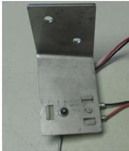
2. Install the fuel level sender bracket inside the tank (note the correct orientation). Ensure that the 'O' rings are installed on the bolts (M6x12mm bolts) on the outside of the tank with the nylock nuts secured from the inside.
